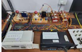
Figure 1: Typical setup connecting CTs/PTs to an industrial relay for line protection.
