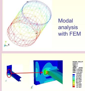
Weld joint stress analyses
